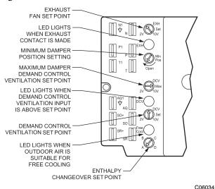
Fig. 76 - EconoMi\$er IV Controller Potentiometer and LED Locations
